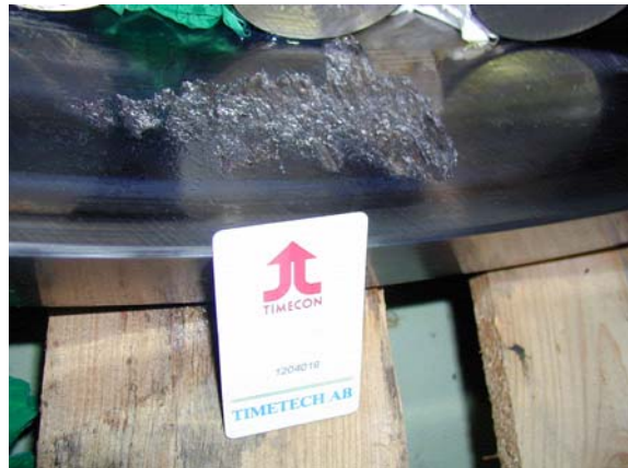
Figure 8. A damage in the bearing outer ring approximately 120 × 60 mm. Rust damage was present on rolls and on the outer ring, indicating that water has entered the bearing casing.
