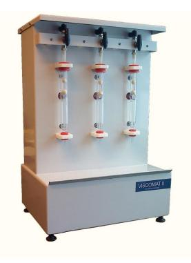
semi-automation strongly reduces operator influence and the time gain is high compared to manual analysis.The system is designed according to and strictly follows the standard test methods ISO 5351 and SCAN-CM 15.
